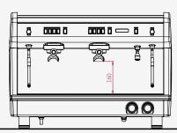
2 Group 3 Group **Colour Options:** Height (mm) 554 554 Width (mm) 768 983 Jet Black Depth (mm) 527 527 Weight (kg) 58 74 **Traffic White** Steam Boiler Size (Litres) 13 20 Coffee Boiler Size (Litres) n/a n/a Group Element (W) **Carmine Red** n/a n/a Steam Boiler Element (W) 3500 (option 4200) 6000 (option 4700) Coffee Boiler Element (W) n/a n/a Total Power (W) 3800 (option 4500) 6300 (option 5000) Voltage (V) 230 (option 400) 400 (option 230)
